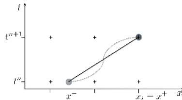
$$\begin{aligned}\frac{dx}{dt} &= v(x, t), & x(0) &= x_0, \\ \frac{d\rho}{dt} &= 0, & \rho(x, 0) &= \rho_0(x).\end{aligned}$$
