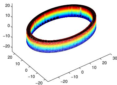
Compute the volume, mass and moment of inertia of the pipe section with respect to the  $y$ -axis using integration. Use elliptical cylindrical coordinates
