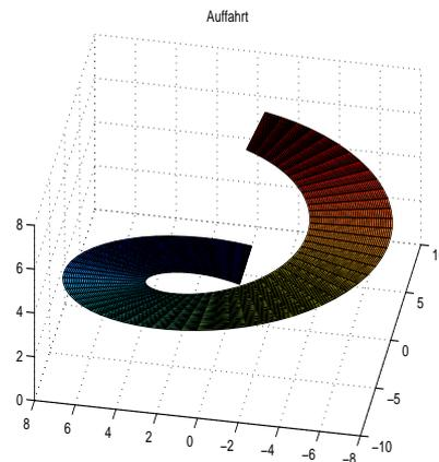
$$\delta p / \delta \phi = \begin{pmatrix} -r \sin(\phi) \\ r \cos(\phi) \\ 1 \end{pmatrix} \quad \delta p / \delta r = \begin{pmatrix} \cos(\phi) \\ \sin(\phi) \\ 0 \end{pmatrix}$$
