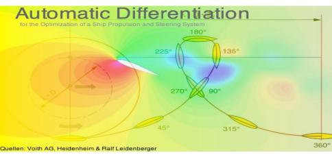
Automatic Differentiation for the Optimization of a Ship Propulsion and Steering System
