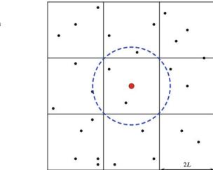
Fig. 3 Fictitious Cartesian grid: neighboring search is done within the nine cells in a two-dimensional space. The smoothing length is constant and the support domain for the particles is 2L
