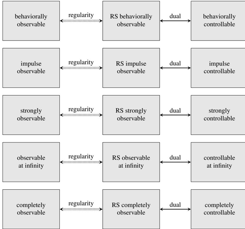
Fig. 2: Illustration of duality between observability and controllability.
