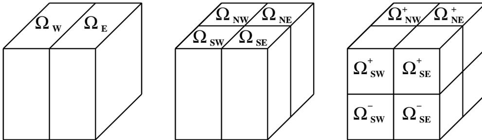
**Fig. 1.** Splitting of the cell  $\Omega$  into eight subcells in three stages.
