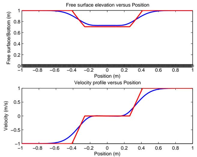
Fig. 4. Semi-implicit SPH scheme rarefaction solution (solid line - blue) versus exact solution (solid line - red). 200 particles is used in the numerical solution.
