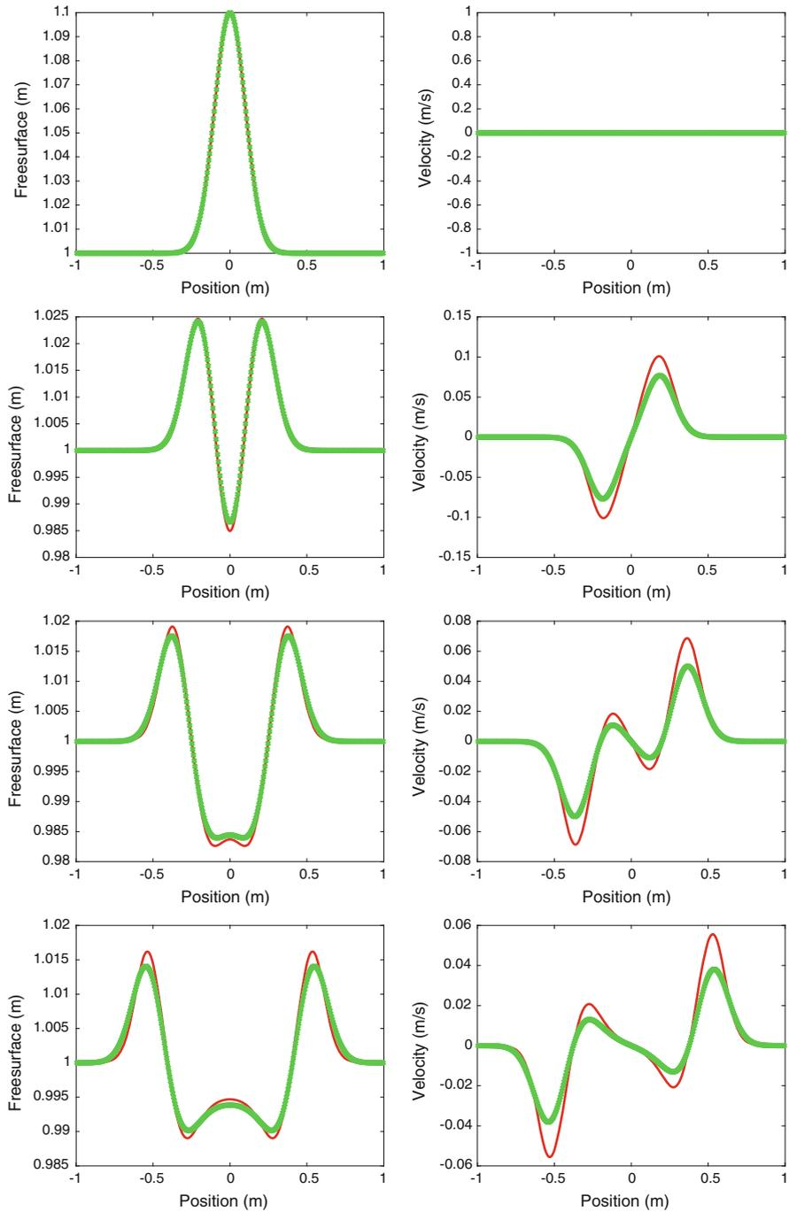
**Fig. 5** Cross section of semi-implicit solution (green) versus reference solution (red): Free-surface (left), velocity (right) in the  $x$ -direction at times  $t = 0.0$  s,  $0.05$  s,  $0.10$  s,  $0.15$  s
