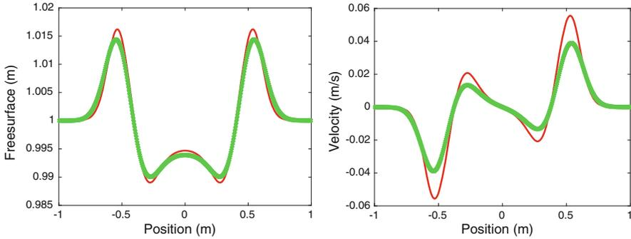
**Fig. 6** Cross section of semi-implicit solution (*green*) versus reference solution (*red*): Free-surface (*left*), velocity (*right*) in the  $x$ -direction at times  $t = 0.15$  s with a higher resolution of 195,496 particles
