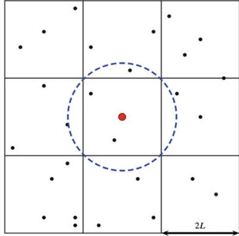
a particle can only interact with particles in its macro cell or in neighboring macro cells. For the two-dimensional case of the present study we only need to loop over the bounding box of nine macro cells (see Fig. 3).
