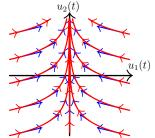
The vector field  $F(x)=(-\frac{x_1}{2},1)$  on  $\mathbb{R}^2$  and some trajectories of the corresponding system  $u_1'=-\frac{u_1}{2},\ u_2'\equiv 1.$
