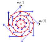
The vector field  $F(x)=(x_2,-x_1)$  on  $\mathbb{R}^2$  and some trajectories of the corresponding system  $u_1'=u_2,\ u_2'=-u_1.$
