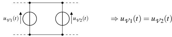
Fig. 15: Parallel interconnection of voltage sources
