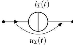
Fig. 8: Symbol of a current source
