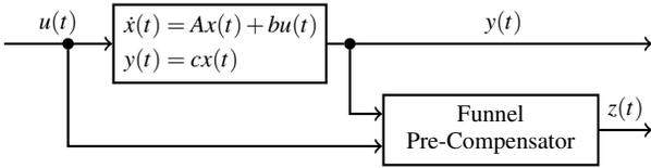
Fig. 2: Interconnection of (1) with funnel pre-compensator (6).
