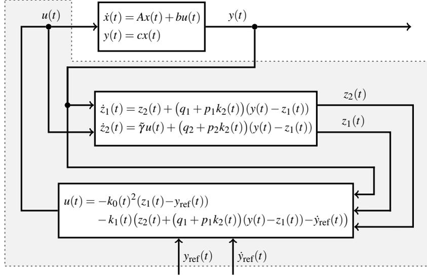
Fig. 3: The funnel controller (10) applied to system (1) consisting, indicated by the grey box, of a funnel pre-compensator (6) and a controller (4).
