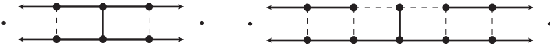
FIGURE 1.2. An ordinary spanning tree of G (left), and a topological spanning tree of G (right)
